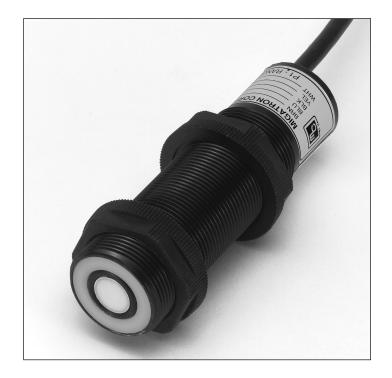
The LED indicator illuminates when the ultrasonic wave from the sensor is reflected back to the sensor within the desired range. The sensor provides precise proximity or level sensing regardless of target color, density or transparency. The sensor is equally effective on liquid, metal, plastic or glass targets.
